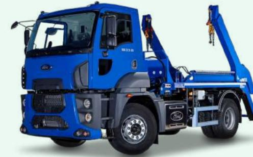
The Skip Loader design to carry containers of uncompactable solid waste has structure which extension arms, too, can be added to according to the need. Stabilization legs (jacks) can be made horizontal or vertical depending on the load state.
