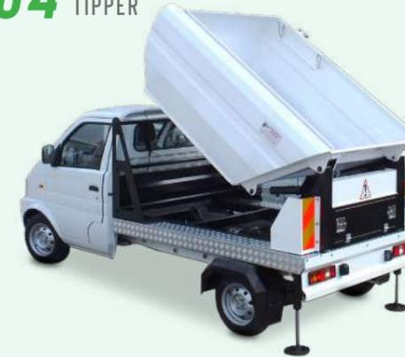
**Maxi Tipper** was made by Timak, 3,5 -6 tone in vehicle group having 4-6m<sup>3</sup> capacity, both have compacting and lifting container system, those vehicles feature small and maeuverability are easy solution for collecting garbage in cities. Because of vehicle cabin entry height is low, provides comfortable use for drivers.
