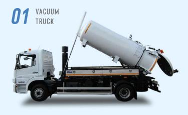
Sewage Trucks are the equipments designed and produced in order to collect the wastes accumulated in reservoirs and sewers by means of suction pump and transport them.
