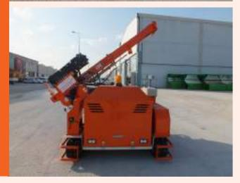
Guardrail pile driver machine is specially designed for driving the highway poles required within the scope of Highway Road Safety precautionary works. It offers a professional solution in accordance with the required power and other features for the installation of signs, barriers and guardrails used on highways.
