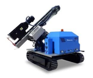
Solar pile driver is a machine used to drive poles into the ground to lay foundation for the solar panel. The vibrating hammer on the vertically movable guides is driven by hydraulic motors powered by the diesel engine on the machine. Vertical vibrations are transmitted to the pile and driving into ground is performed, while horizontal vibrations are damped to ensure stable operation of the machine.
